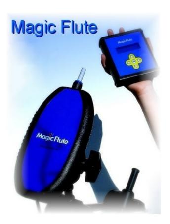
The Magic Flute is not only an instrument but also acts as the remote control for the Control Module (sip & puff).
