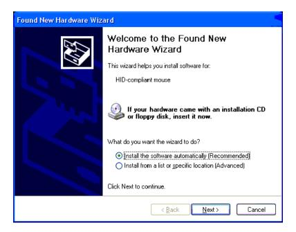
Click on "Install the software automatically" and then click "Next". Windows will automatically install the Human Interface Device (HID) driver.
