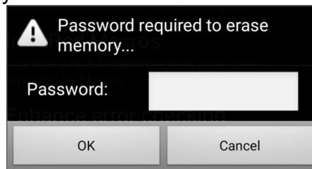
After you have entered the password a progress bar will display the erase process. First the 250 single InfraRed signals are erased (these are stored in 8K blocks).
