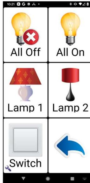
3. Make a long click on the command you want to use. The familiar Command dialog will appear allowing you to edit the cell and record infrared signals etc. with two additional entries to allow you to control your Z-wave devices: **Control Z-wave device** and **Run Z-wave scene**.
