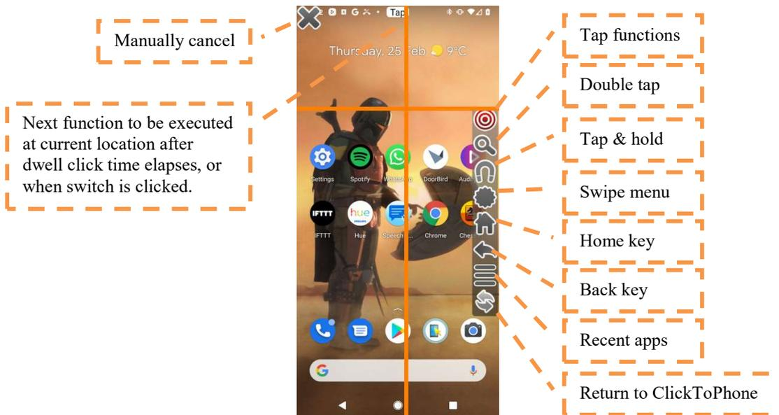
When you move the mouse pointer over the swipe menu soft key then a sub-menu of arrows will appear. Move the mouse pointer over the direction you want. With the direction highlighted, move the crosshairs to the location where you want to perform the swipe. Then press your switch to perform the swipe.
