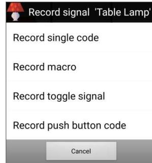
There are four options associated with recording infrared signals. **Record single code**, **Record macro**, **Record toggle** and **Record push button code**. For now choose **Record single code**. You will be prompted to check the brand of remote control you are recording from.
