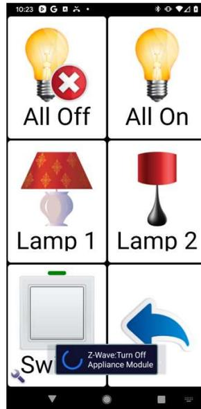
**Note:** ClickToPhone only supports two Z-wave devices types directly. Appliance modules (including light switches and relays) and Dimmer modules. If you want to control a device belonging to another device category then you must first create a scene that turns it on or off. Then you can run the scene as described in the following section to turn on or off the device.
