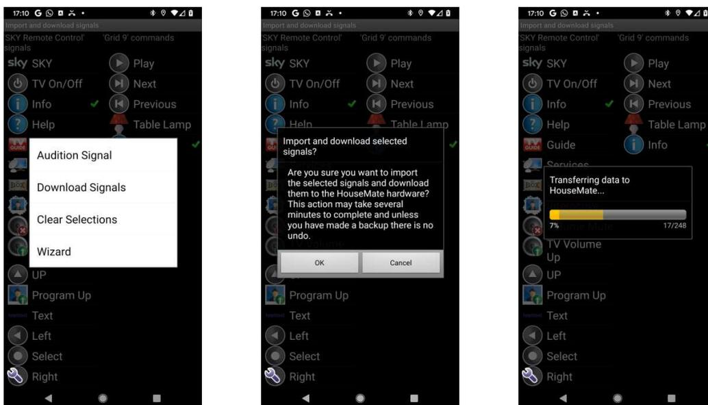
You can make more than 1 pairing. To download the signals press the spanner symbol and choose **Download Signals**. The InfraRed signal data will be transferred into the HouseMate memory. When the transfer has completed you can test the commands by clicking on them.
