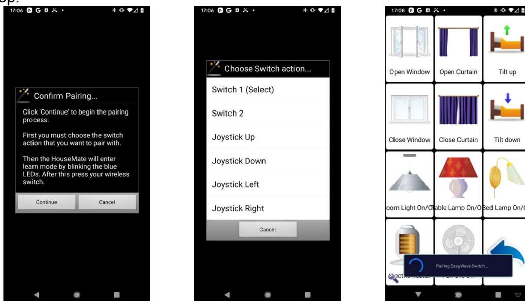
Ensure that the pairing has been successful by pressing the switch and confirming that the desired switch action occurs.
