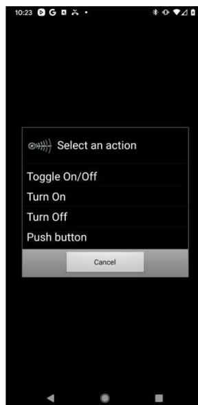
6. Choose an action. After you have chosen it confirm that it operates as required by clicking the command. A short popup dialog should confirm the action that is being performed on the device.
