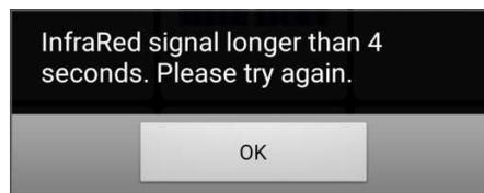
Another mistake is to press the HouseMate button and the remote control button at the same time. It is important to press and hold the HouseMate button before you press the remote control button so as to capture all the signal. You can leave as long as you want between pressing the HouseMate button and pressing the remote control button with no fear of using up memory because HouseMate only starts the recording process when it starts to receive an InfraRed signal.
