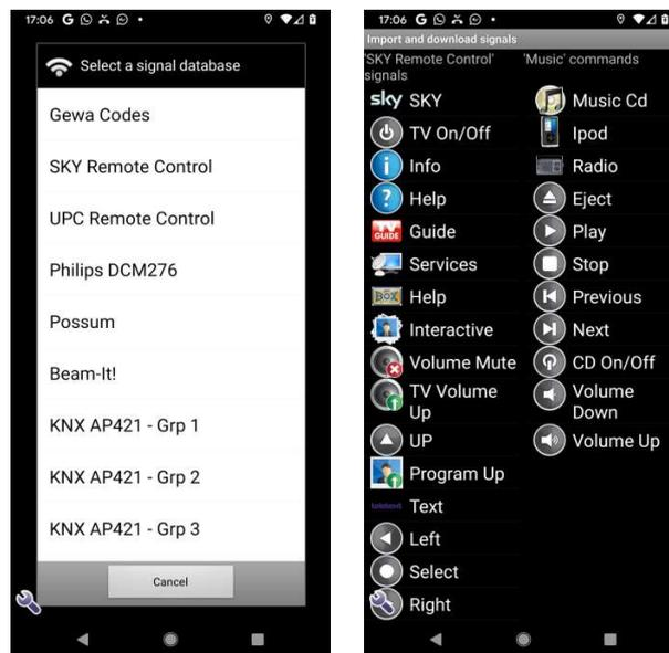
The left-hand list contains the signals stored within the database and the right-hand list contains the commands defined within the current grid. Pair the signal you want to download with the chosen command in the grid. In the example below we have paired the **Info** signal in the SKY remote database with the **Info** command in Grid 10.
