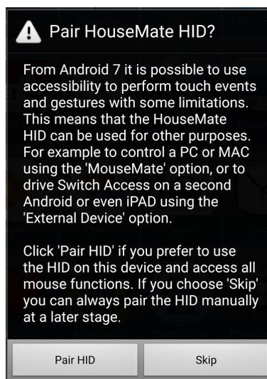
From Android 7 it is possible to use accessibility to move the cross-hairs and perform gestures on the screen. This frees up the HouseMate HID which can be used to control a remote PC, MAC or another Android or iOS device using the MouseMate function. There are, however the following limitations in using accessibility alone to control the screen:
