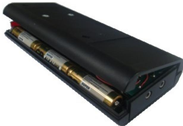
TwoXTen viewed with the back-cover slightly open on the left hand side. Note how the cover is hinged on the right hand side. Always open the cover from the left hand side.
