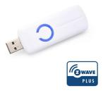
The button on the stick can be used to add or remove devices from the network. Press once to enter inclusion mode (blue LED). Press and hold for exclusion mode (flashing yellow LED). The unit is powered by an internal battery charged by USB.
