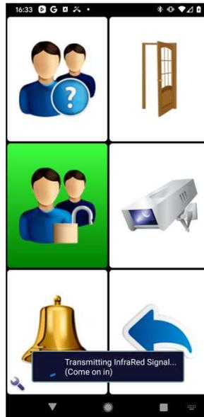
**Tip:** The bell symbol in this default grid is InfraRed command 1, and as such will trigger the output relay in your HouseMate hardware, transmit an EasyWave or Z-Wave signal if fitted. You can copy this command to the homepage and use it to call for assistance at any time. See Chapter 25 for further details on hardware related assistance calls.
