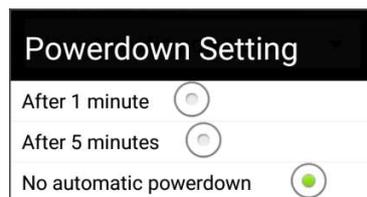
When set to 1 or 5 minutes the HouseMate hardware will automatically switch off if you have not made any switch presses for the chosen time. This allows the phone to turn off the screen and go to sleep and conserves the battery life of both units.
