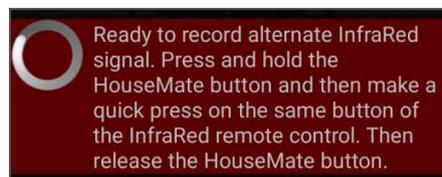
6. Now HouseMate is ready to record a second copy, or alternate, of the signal. This is how HouseMate records the toggle codes described earlier. As before press and hold the button on the HouseMate hardware. Then make a short press of the button on the remote control whose signal you want to record and then release the HouseMate button. While you are doing this the dialog text should change to “**Recording alternate InfraRed signal...**” and HouseMate should beep more rapidly.
