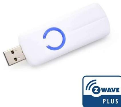
The button on the stick can be used to add or remove devices from the network. Press once to enter inclusion mode. Press and hold for exclusion mode. The unit is powered by an internal battery charged by USB.
